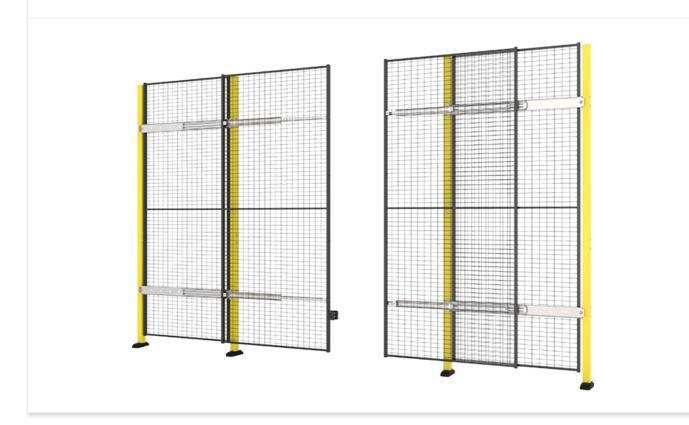
The X-Guard single sliding door without rail with center lock is the optimal safety solution for industrial environments requiring unrestricted height clearance. Designed for handling large goods, this door allows transport via overhead cranes or forklifts. With an opening width of up to 2x2900mm and a maximum height of 2300mm, it provides a spacious and flexible access point.
