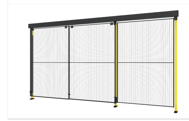
The X-Guard double telescopic sliding door is designed for industrial environments where a large opening is needed, but space is restricted to the side and front, e.g in connection to a vehicular routes. Instead of sliding fully outward, its overlapping panels move along a 2-step rail system, reducing the required clearance. With a maximum width of 2x1500 mm and a height of 2500 mm, it provides efficient access while maintaining a compact footprint.
